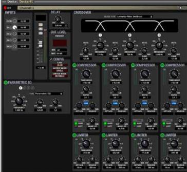
NXA 4BC (4 band compressor/limiter) is a dedicated software and firmware version for the NXA series, tailored for applications where a strict SPL (Sound Pressure Level) limit must be guaranteed.
