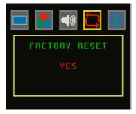
Select YES to return the unit to the factory settings. The default Factory Setting for Video display is 'Full Screen' (1280×720@60Hz), Color setting's factory default rate is the same as shown on the OSD and SDI audio is 'AUTO'.
