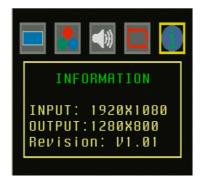
Displays the source input format, the output display format and the unit's software version.
