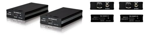
The PRO-HDMIFO-KIT is a Transmitter and Receiver set for sending HDMI signals over long distances via Fiber Optic cabling. Connect a HDMI source to the Transmitter unit and the uncompressed signal will be passed over fiber optic to the Receiver where it is outputted as HDMI for connection to the display. HDMI Transmission distances of up to 300m can be achieved using this advanced fiber optic technology.
