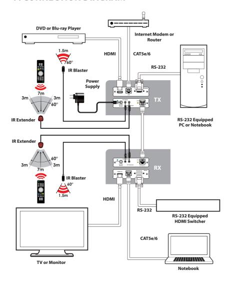
**Note:** Only one of the units need to be connected to power, either the transmitter or receiver, on order for both to operate. In this example the transmitter is powering the receiver
