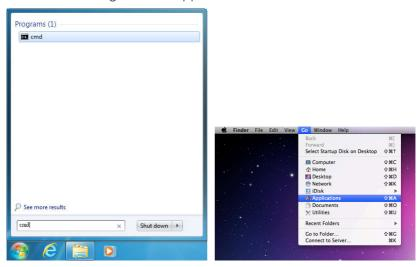
Once in the command line interface (CLI) type "telnet", then the IP address of the unit and port "23" and hit enter.
