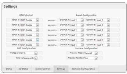
Click on Network Configuration to set the device's IP configuration. Once the changes are saved the system will reset the IP address on the device automatically and user will need to re-enter the IP address to continue the Web GUI function.
