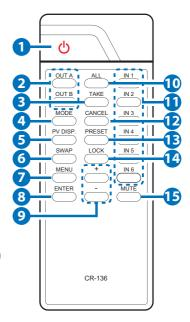
**Select to VIEW ALL:** Press from INPUT 1~6 or MUTE to select input sources for main channel.
